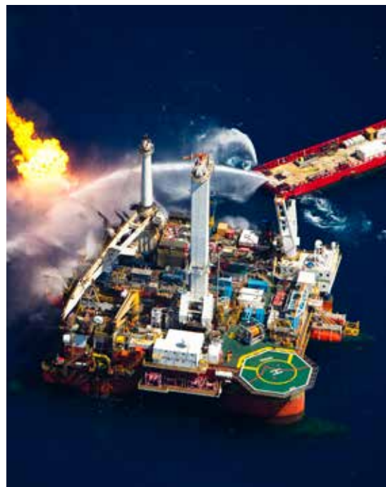
The Q4000 multi-purpose oil field intervention vessel, burns off material from the Deepwater Horizon wellhead near the disaster site in the Gulf of Mexico. ©Daniel Beltrá/Greenpeace
