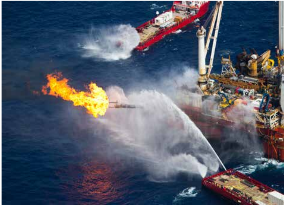
The Q4000 multi-purpose oil field intervention vessel, burns off material from the Deepwater Horizon wellhead near the disaster site in the Gulf of Mexico. ©Daniel Beltrá/Greenpeace
